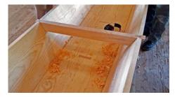
Unlike Western boat building techniques, no caulking or sealants are used in the construction, requiring the careful preparation of tight-fitting joints. This is accomplished by a technique called *Suriawase* (saw fitting), in which the adjacent faces of the assembled joints are sawn together using pull saws, providing matching, gap-free joints. Keel and the side-to-keel joints are prepared this way.
