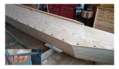
As shown in the photo, the planking which comprises the sides of the boat is attached to the keel and transoms with hand forged steel nails. The wooden components are left unfinished.
